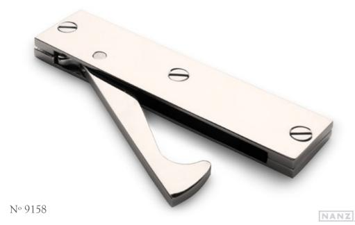
The No 9158 knife-edge pull, which is mortised into the edge of a single or double door, is ideal when a minimum of hardware is required. When the door is closed, only the  $5/16\mathbb{I}$  wide edge is visible. It measures 4-1/4" x 5/16" with a depth of 3/4" or 1". Finished to order in a wide range of finishes.
